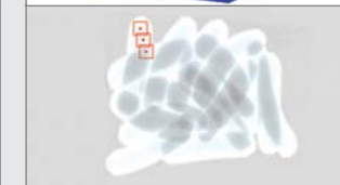
Evolved image processing The background product effect is further reduced enabling foreign bodies to be identified
